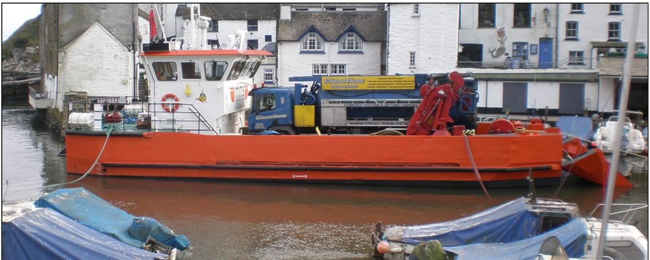
Inner harbour sewer refurbishment works – 60t landing craft complete with lorry-mounted tanker and jet / vac unit on board
