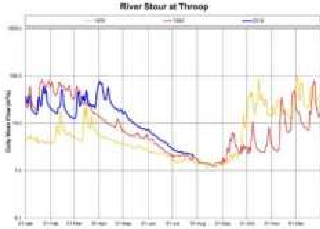
Figure A2.9: Example assessment of river flow – River Stour at Throop 6
